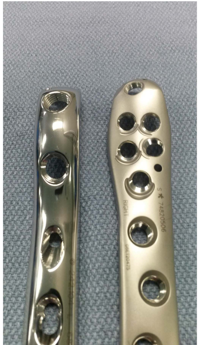
FIGURE 2. Photograph demonstrating geometry of proximal end of PFLP: PFLP on the left was prone to fail compared with plate on the right. Editor's Note: A color image accompanies the online version of this article.
